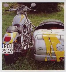
sidecar weight did require some brake modifications. Brembo brakes were added for extra stopping power, and they work very well.
